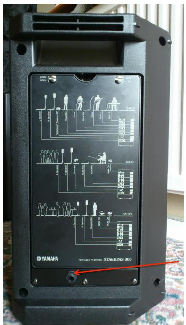
To access the leads needed for the PA, you need to use a coin on the back of this speaker. Inside here are 2 jack leads (ones with a single 'pin') and the 'kettle' lead (to plug into the mains).
