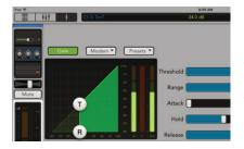
In this example the gate has been switched on and has been set around -50db, so sounds quieter than -50db will be cut off. This is too extreme. If we use a gate (e.g. to stop buzz on a bass guitar or to stop loud squeals called 'feedback'), set the cut off to -70db by using the threshold and range controls. Keep the release 'long'. We may use a gate on some drums if we get feedback between two drums or if a 'low tom' starts 'rumbling'!
