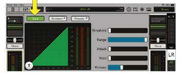
On the left we can see that the 'Gate' is in the shape of a triangle. In this example, the gate is not on and therefore won't cut out any of the quieter sounds or buzzes.
